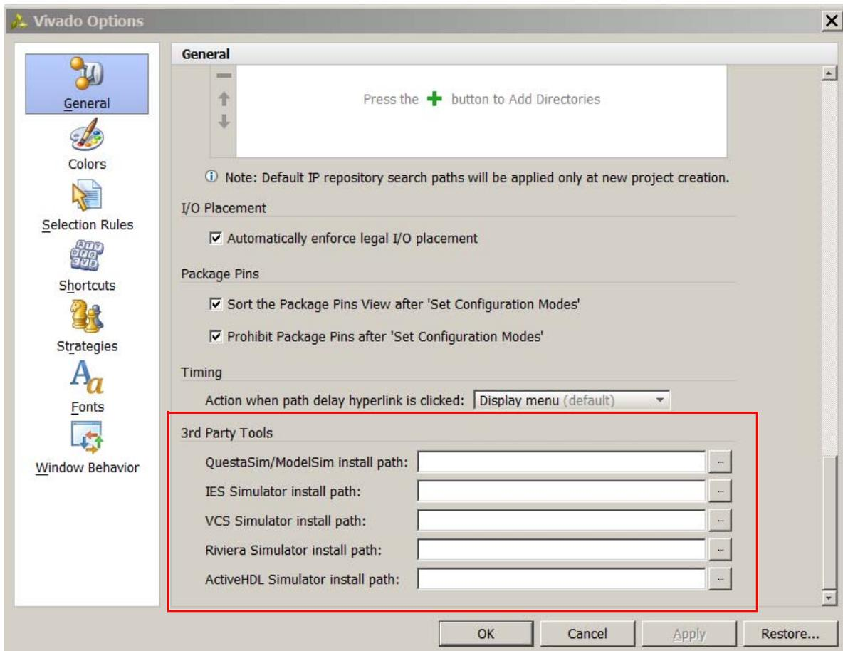
Figure 8-1: Vivado Design Suite General Options, Install Path
