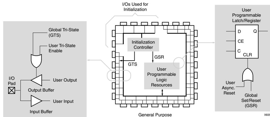
Figure 6-1: Built-in FPGA Initialization Circuitry Diagram
