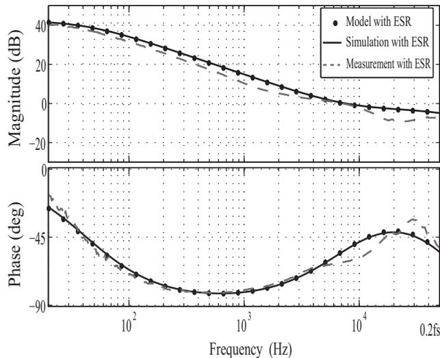
Fig. 12. Comparison control-to-output transfer  $T_{co}(s)$  with simulation, measurement and model ( $R_L \rightarrow \infty$ ).
