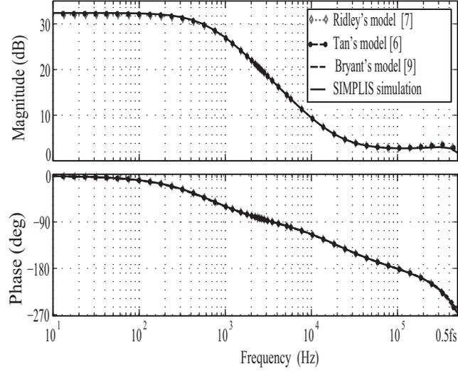
Fig. 3. Comparison of the Ridley [7], Tan [6] and Bryant [9] models control-to-output transfer  $T_{co}(s)$  with SIMPLIS simulation for a PCMC boost converter with resistive load ( $50\Omega \parallel 10\mu\text{F}$ ).
