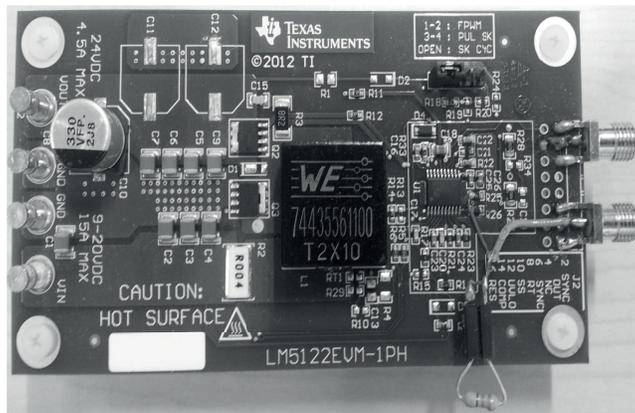
Fig. 11. Modified LM5122EVM-1PH synchronous boost controller evaluation module
