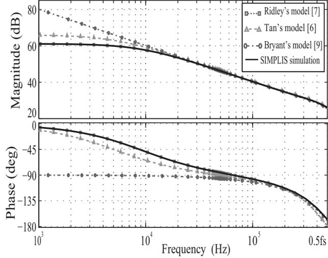
Fig. 4. Comparison of the Ridley [7], Tan [6] and Bryant [9] models control-to-output transfer  $T_{co}(s)$  with SIMPLIS simulation for a PCMC boost converter with capacitive load ( $26\text{nF}$ ).
