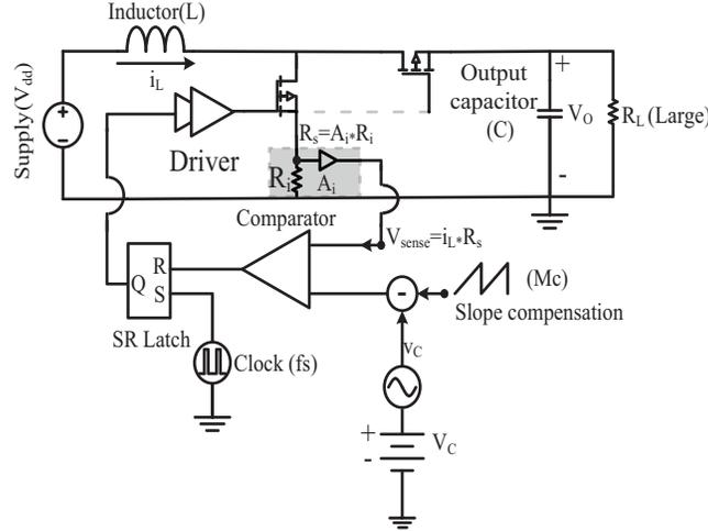
Fig. 5. A closed-current loop PCMC based boost converter with RC ( $R_L \parallel C$ ) load
