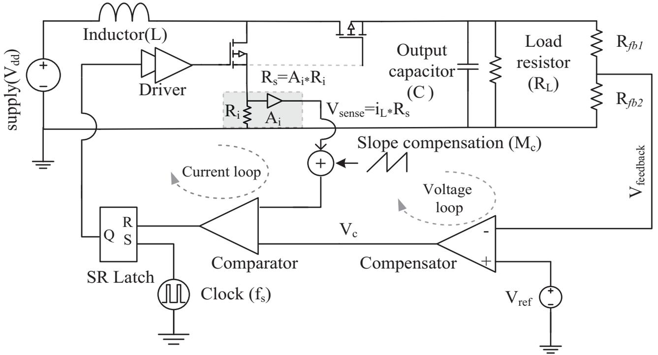
Fig. 1. A peak current-mode control based bi-directional boost converter
