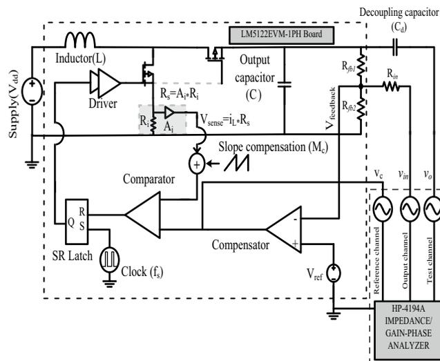
Fig. 10. Measurement schematic of a peak current-mode control based bi-directional boost converter with capacitive load ( $370\mu\text{F}$ )
