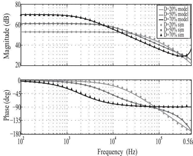
Fig. 9. Effect of duty cycle variation on the dominant pole location for a capacitive load
