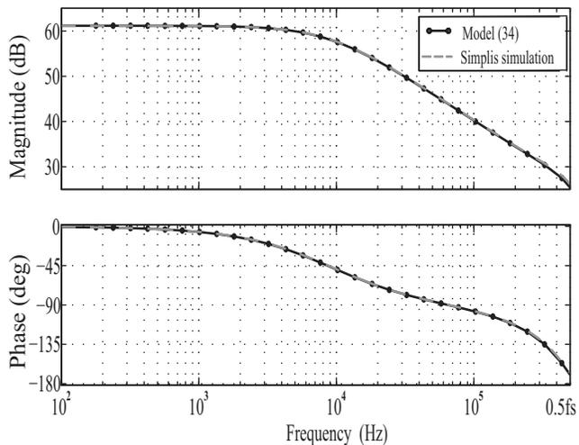
Fig. 8. Control-to-output transfer  $T_{co}(s)$  according to model (34) and SIMPLIS simulation for capacitive load ( $R_L = \infty$ ,  $C=26\text{nF}$ ).
