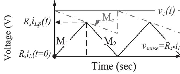
(a) Continuous-time domain converter waveform for PCMC
