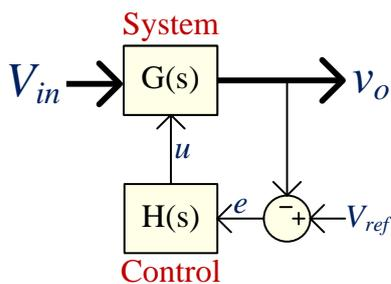
Fig. 7.1. Basic block diagram of a closed-loop control system
