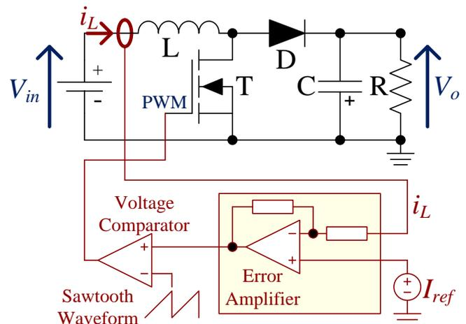
Fig. 7.10. An inner average current loop of a boost converter
