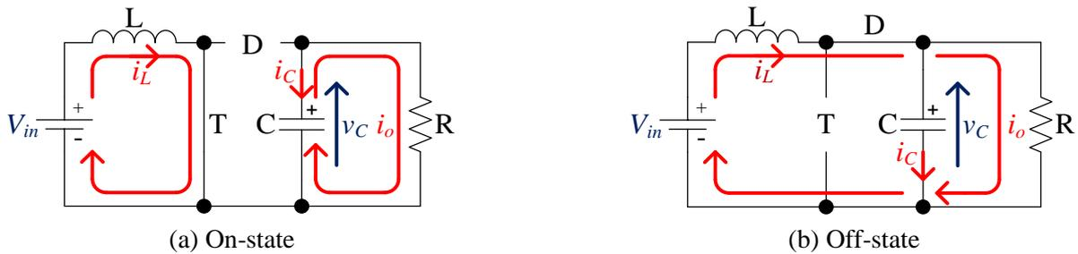
Fig. 7.5. Equivalent circuits of a boost converter in Continuous Mode
