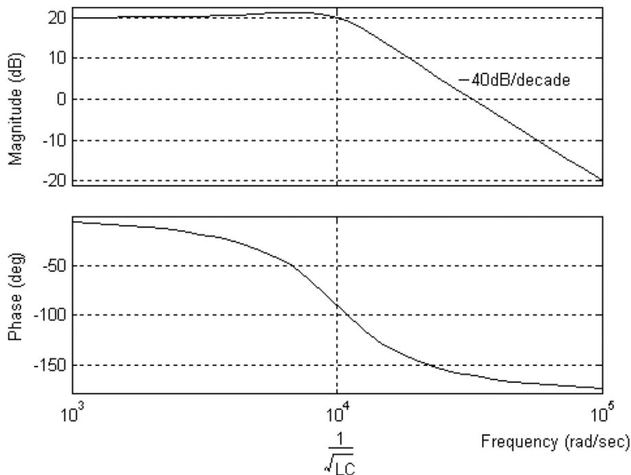
Fig. 7.4. Bode plot of a small signal transfer function (duty ratio to output voltage) of a buck converter in continuous mode
