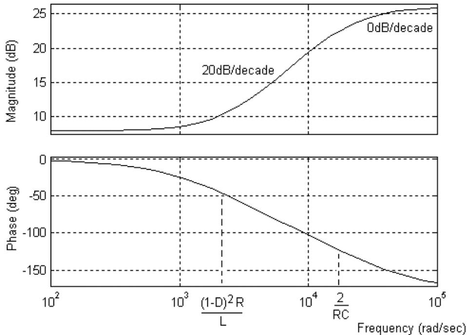
Fig. 7.13. Bode plot of a boost converter with inner current loop
