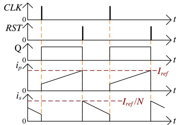
Fig. 7.12. Idealised waveforms of a current loop of a flyback converter with peak current mode control
