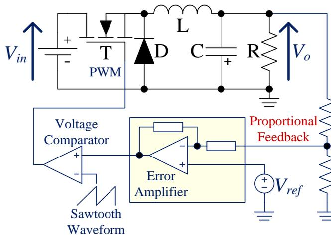
Fig. 7.9. A typical voltage mode control system of a buck converter
