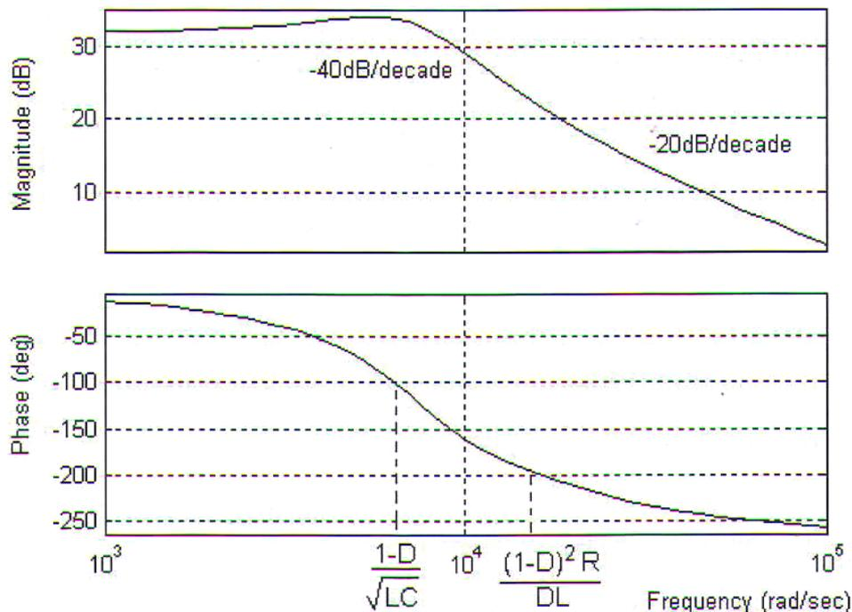
Fig. 7.8. Bode plot of a small signal transfer function (duty ratio to output voltage) of a buck-boost converter in continuous mode
