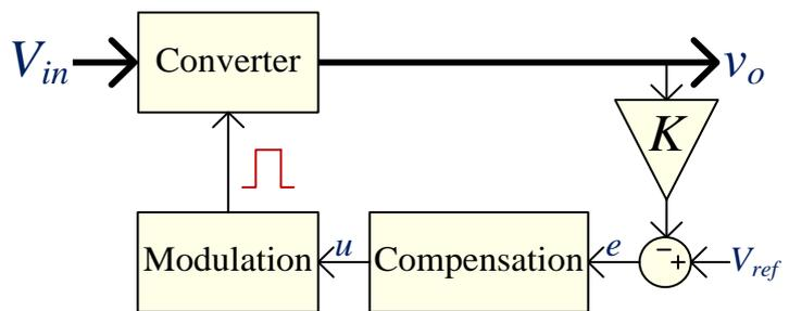
Fig. 7.2. Block diagram of a signal loop voltage controlled DC/DC converter
