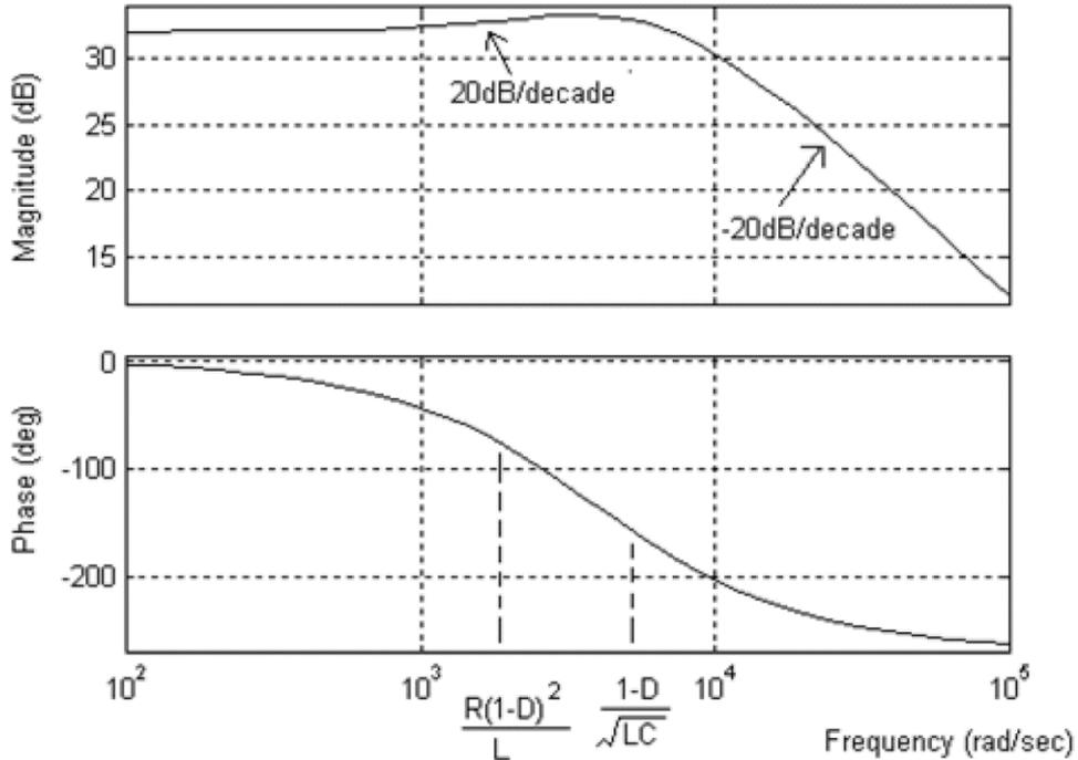
Fig. 7.6. Bode plot of a small signal transfer function (duty ratio to output voltage) of a boost converter in continuous mode
