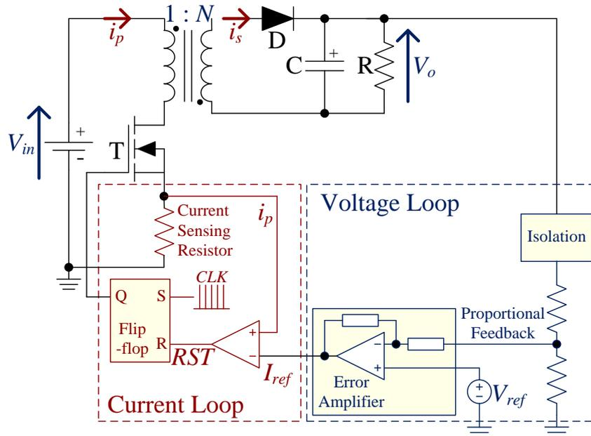
Fig. 7.11. A flyback converter with peak current mode control
