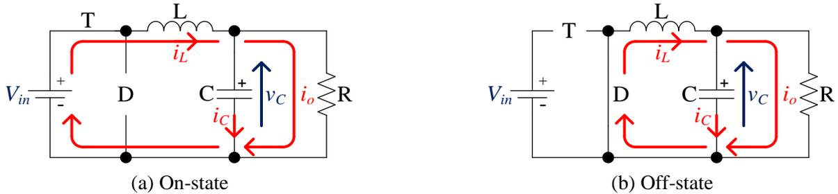
Fig. 7.3. Equivalent circuits of a buck converter in continuous mode
