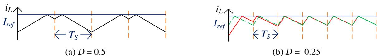
Fig. 7.14. Inductor current waveforms under peak current mode control
