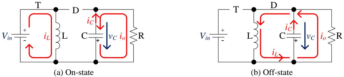
Fig. 7.7. Equivalent circuits of a buck-boost converter in continuous mode
