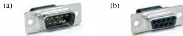
Figure 13.35: Nine-pin “D-sub” RS-232 connectors: (a) male; (b) female. Top-row pins number 1 to 5 (LR), bottom-row pins number 6 to 9 (LR).
