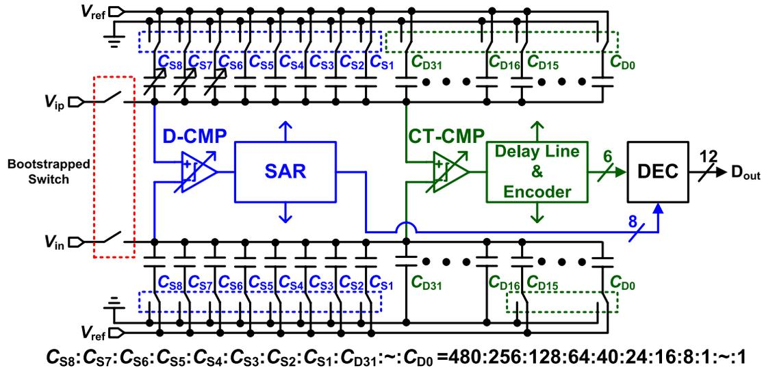
Fig. 5. Block diagram of the proposed 12 bit SAR-assisted digital-slope ADC.
