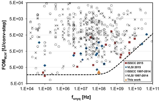
Fig. 17. Comparison of Walden FoM with the ADCs presented at ISSCC and VLSI between 1997 and 2015 [23].
