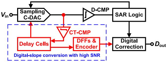
Fig. 3. Block diagram of the proposed SAR-assisted digital-slope ADC.
