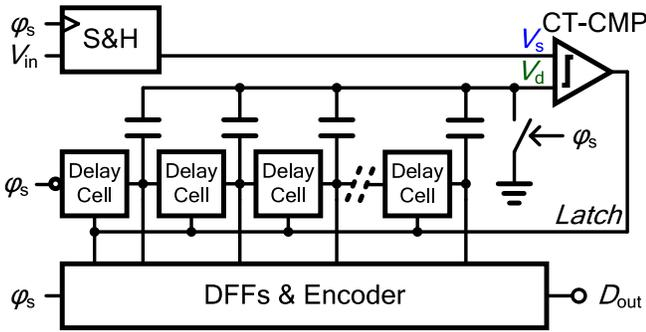
Fig. 1. Block diagram of an asynchronous digital-slope ADC.
