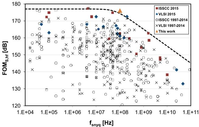
Fig. 18. Comparison of Schreier FoM with the ADCs presented at ISSCC and VLSI between 1997 and 2015 [23].
