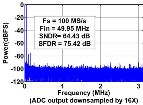
Fig. 15. FFT plot with input frequency close to Nyquist frequency.
