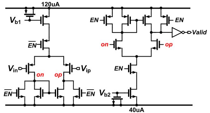
Fig. 6. Schematic of a low-noise low-power CT-CMP.
