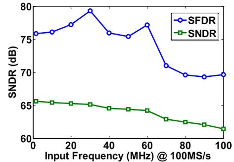
Fig. 14. Measured dynamic performance versus input frequency at 0.9 V and 100 MS/s.
