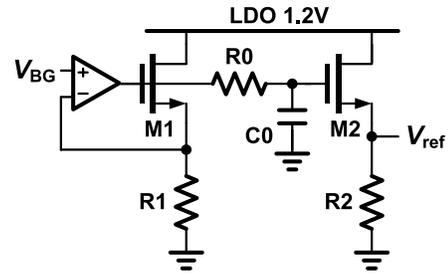
Fig. 11. Schematic of reference buffer.
