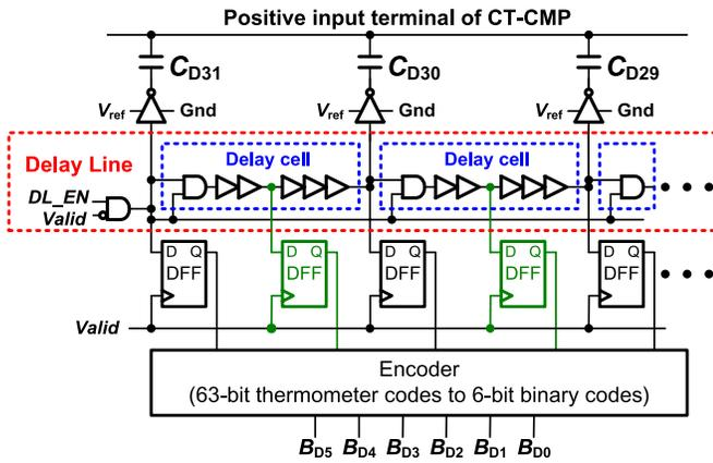
Fig. 8. Implementation of the 6 bit digital-slope fine ADC.
