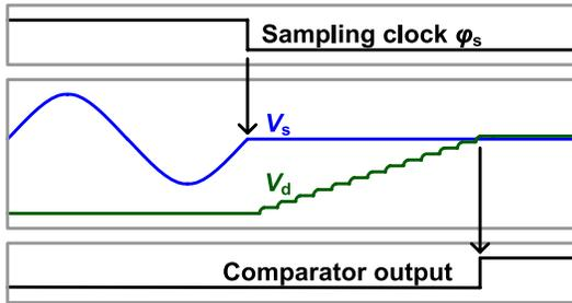
Fig. 2. Timing diagram of a digital-slope ADC.
