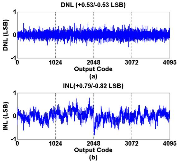
Fig. 13. Measured static performance. (a) DNL. (b) INL.
