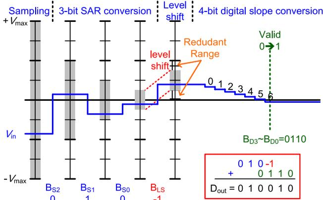
Fig. 4. A 6 bit operation example of the proposed SAR-assisted digital-slope ADC.
