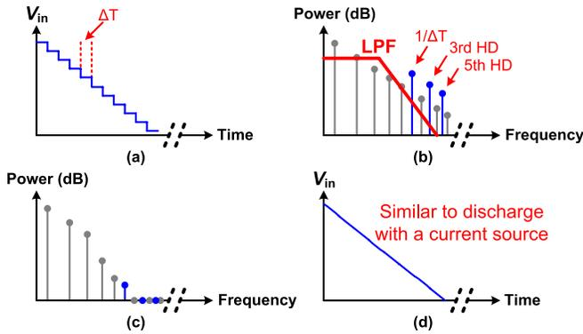
Fig. 7. (a) Stair step curve with an interval of  $\Delta T$ . (b) FFT spectrum of the stair step curve. (c) Effective spectrum after filtering by the low-bandwidth CT-CMP. (d) Equivalent input signal curve of the low-bandwidth CT-CMP.
