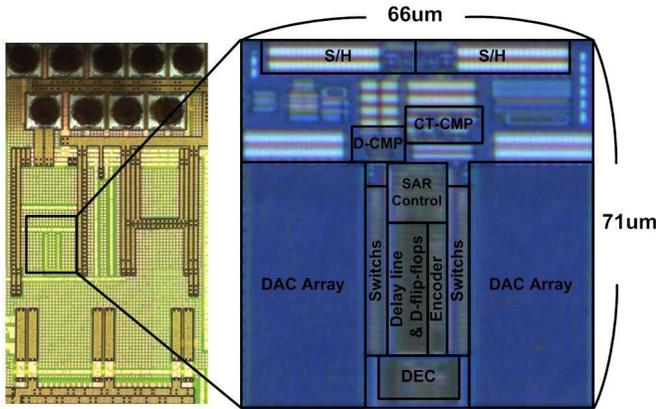
Fig. 12. Chip micrograph and delayed zoomed-in view of ADC core.
