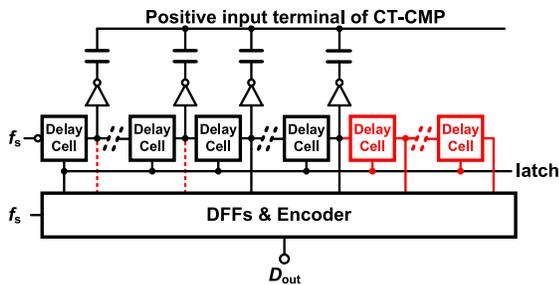
Fig. 10. Implementation of latency compensation.
