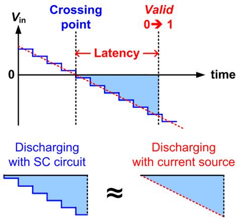
Fig. 9. The latency from the input crossing point to the *valid* signal generation.
